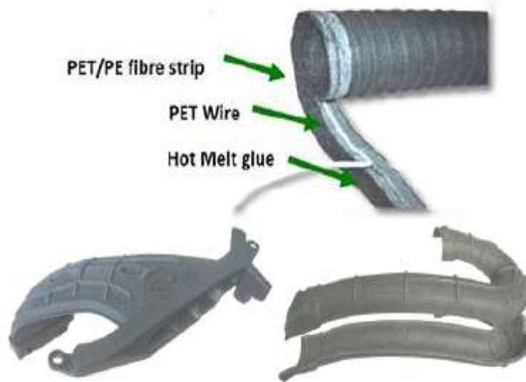
Figure 1: Porous type duct of intake system
